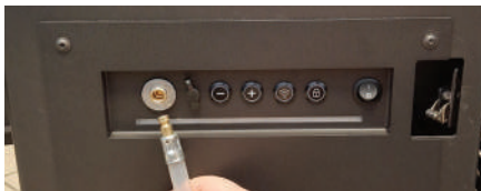
Fig. 27 Quick-connect fuel filler with matching external pump connector
