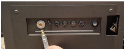
Fig. 28 External pump power connector with matching plug from the external pump
